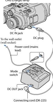
The CHG (charge) lamp lights up and charging starts. The CHG (charge) lamp turns off when the battery pack is fully charged.
